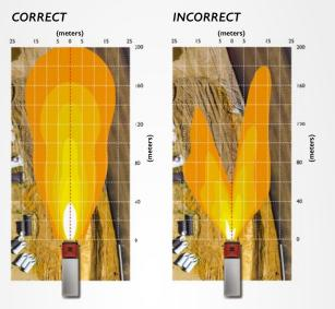
**Off-road illumination.** To ensure optimum visibility when working with your headlamps on, your headlamps need to be positioned correctly such as to provide an intense and precise source of luminous power – this is the only way to guarantee your comfort and safety while also taking the stress out of driving.
