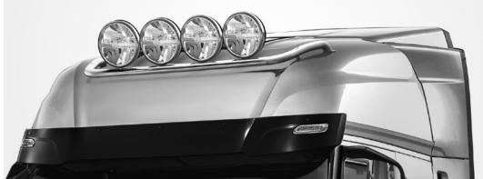
**SKY LIGHT High roof.** With LED cable for 6 lights, 6 fixed type holders, 5 white LEDs. Stainless steel, 60 mm.
